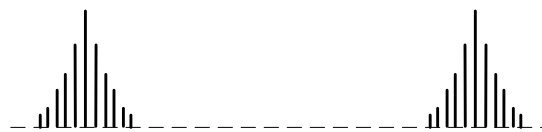
Figure 5. Amplitude Compression and Extension For Phase Coincidence Pulse
