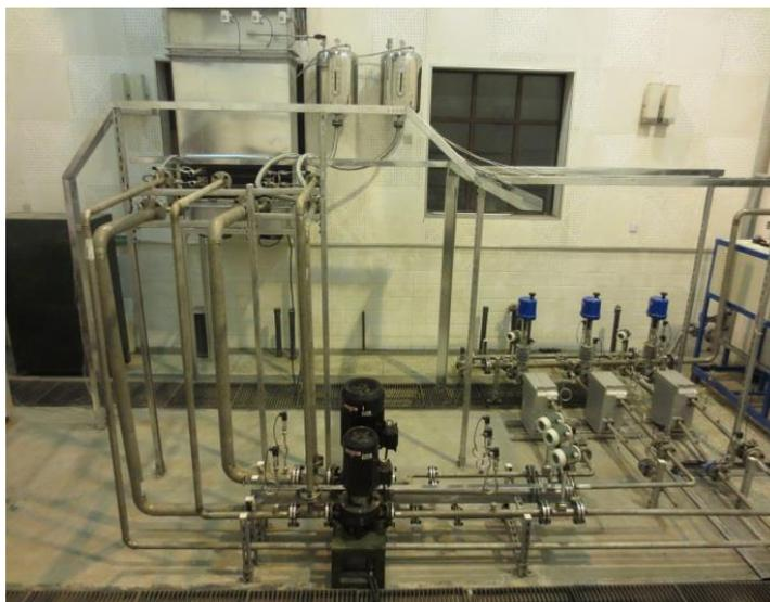
Figure 8. Cooling System Test Bench
