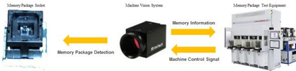
Figure 6. MVMS Operating Control Structure
