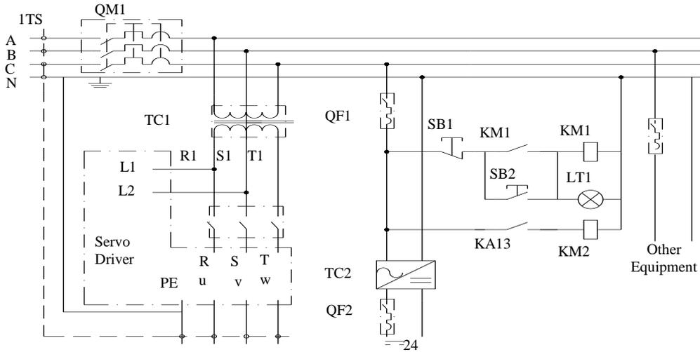
**Figure 5. The System Main Wiring Diagram**
