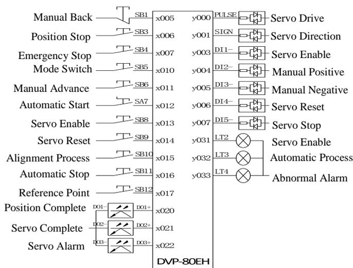
**Figure 6. Input and Output Port Assignment Map of PLC**
