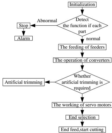
**Figure 3. The Control System Flow Chart**
