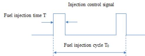
**Figure 11. ECU Fuel Injection Control Signals**
