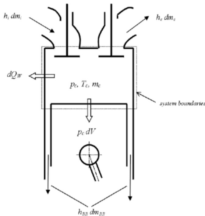
Figure 1. Energy Balance in the Cylinder
