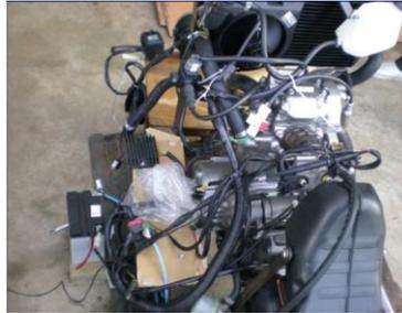
**Figure 13. Engine Installed In FSAE**
