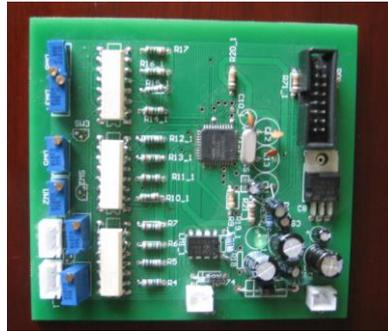
**Figure 14. The Intake Air Correction Control Unit**
