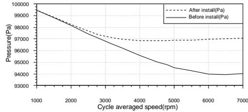
**Figure 5. The Changes of Pressure in Intake Pressure Sensor with Engine Speed**
