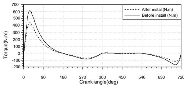
Figure 4. Torque Changes at the Maximum Speed of 5000 RPM
