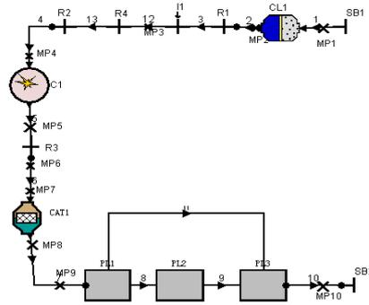
Figure 2. FSAE Car Engine Cycle Simulation Model in BOOST
