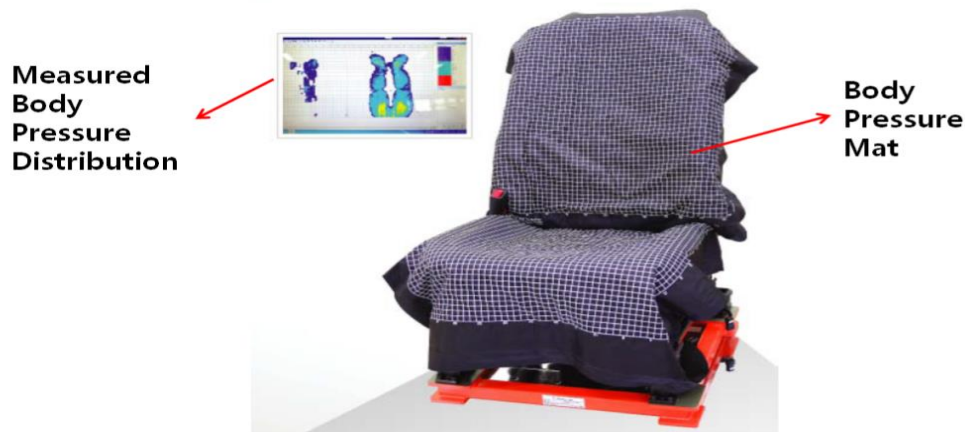
Figure 6. Body Pressure Distribution Test
