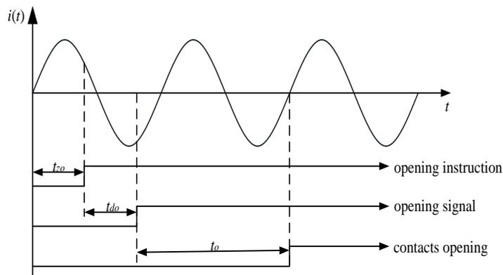
**Figure 2. Sequence Diagram of Circuit Breaker Opening**
