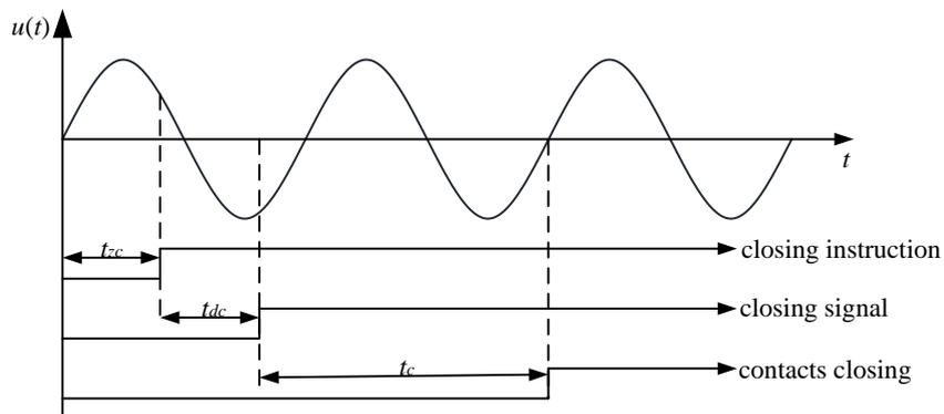
**Figure 1. Sequence Diagram of Circuit Breaker Closing**
