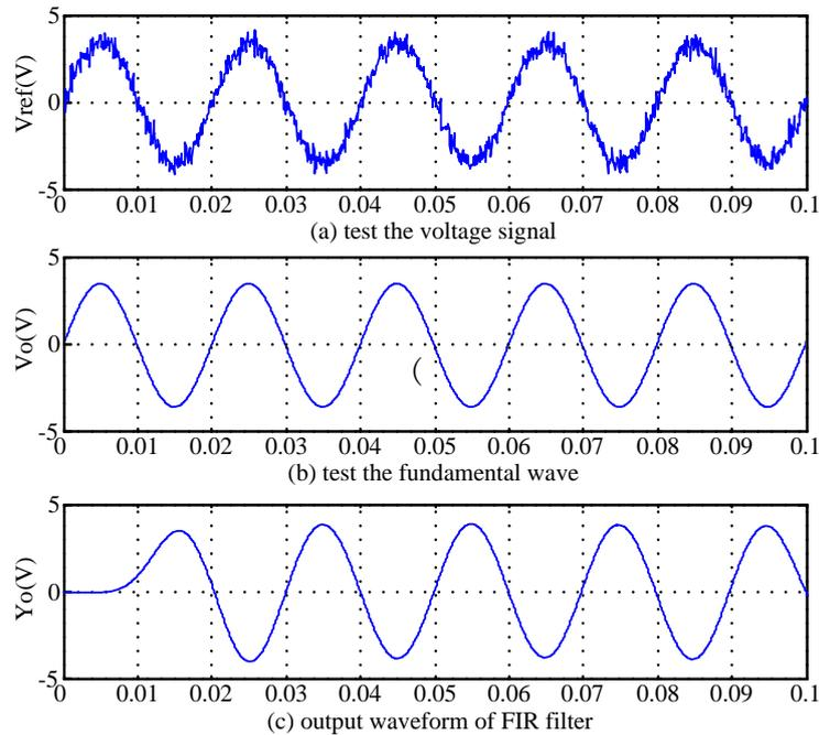
**Figure 5. Filter Test Results**
