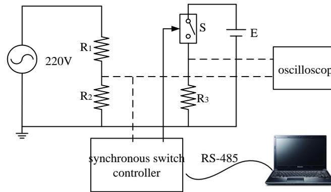
**Figure 7. Accuracy Test Device of Synchronous Controller**
