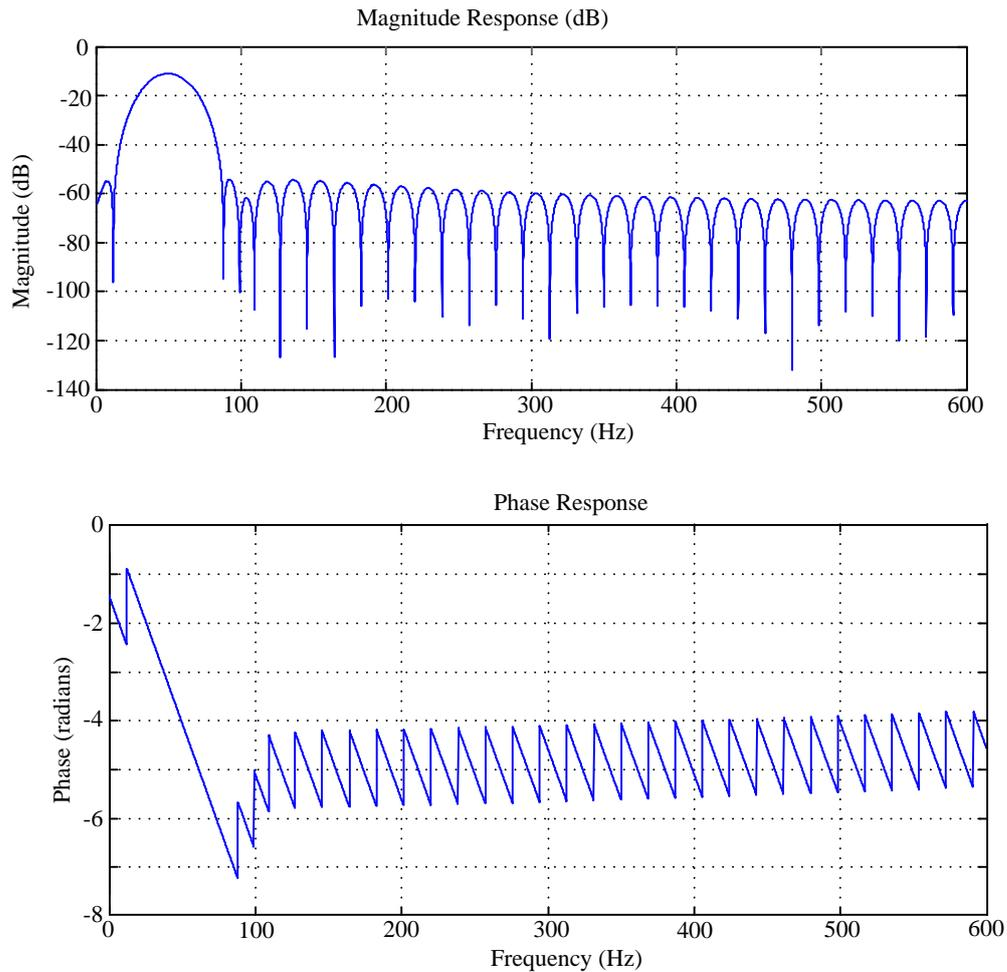
**Figure 4. Frequency Response of Band-Pass FIR Filter**
