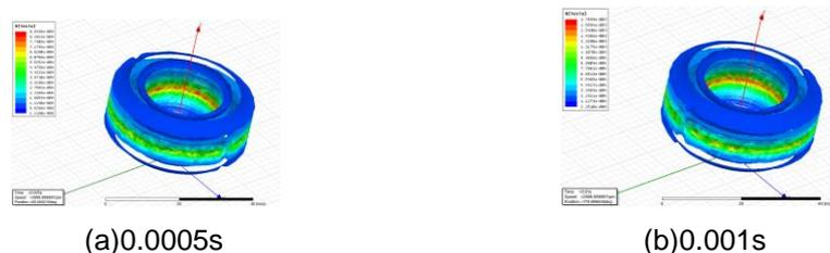
**Figure 10. Coaxial Windings Type Topology Simulation Scalar on the Magnetic Induction Intensity**
