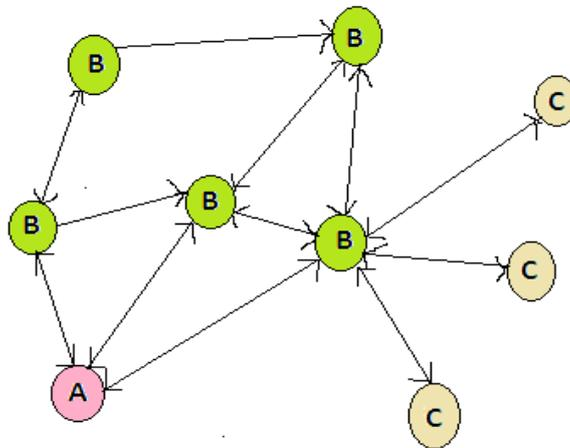
**Figure 1. Mesh Topology Network**
