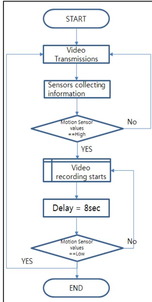
**Figure 9. Algorithms of Infrared Camera and Mainboard**
