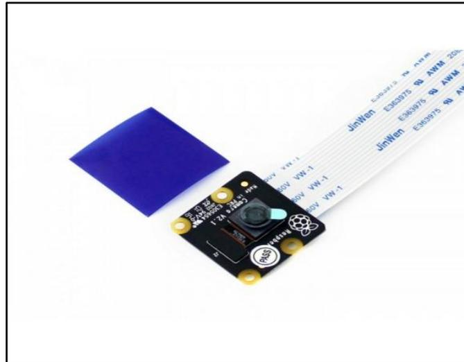
**Figure 3. Infrared Camera**
