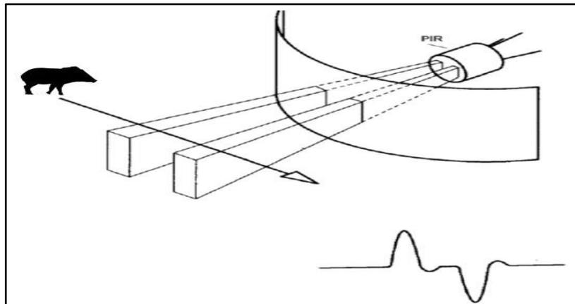
**Figure 4. PIR Sensor Operating Principle**
