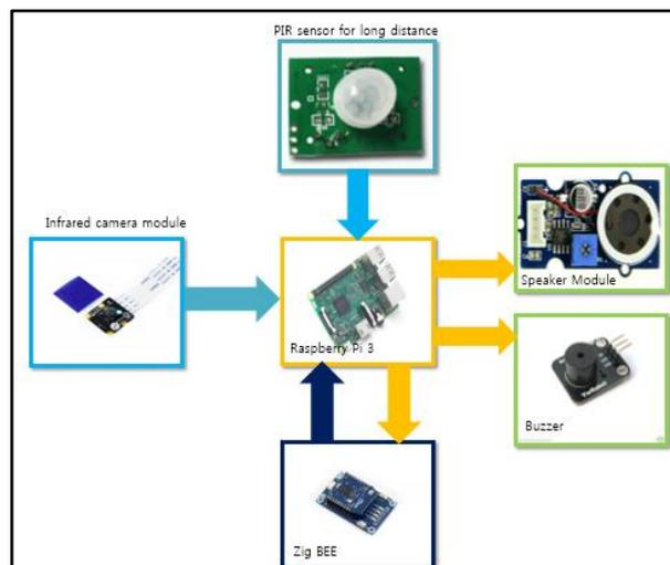
Figure 6. An Overall Configuration Diagram
