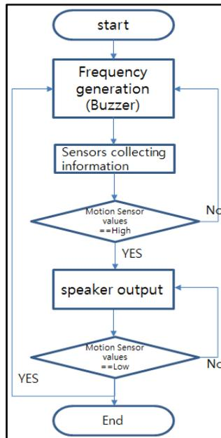
Figure 12. Ultrasound and Buzzer Output Algorithm
