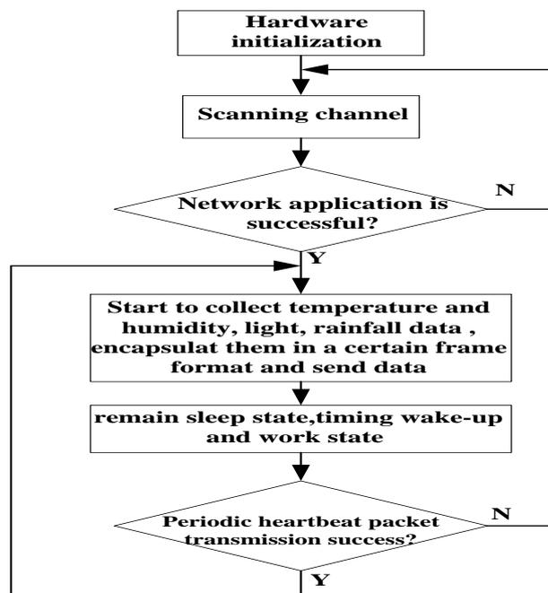
**Figure 5. Software Program Flow Chart of the Terminal Node**
