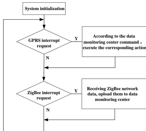
**Figure 4. Main Program Flow Chart of the Gateway Node**
