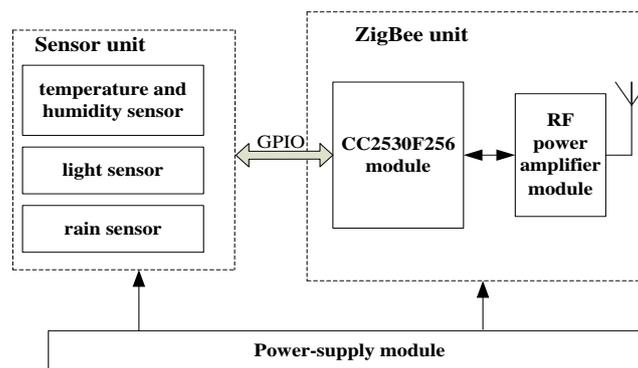
**Figure 3. Hardware Structure Diagram of the Terminal Node**
