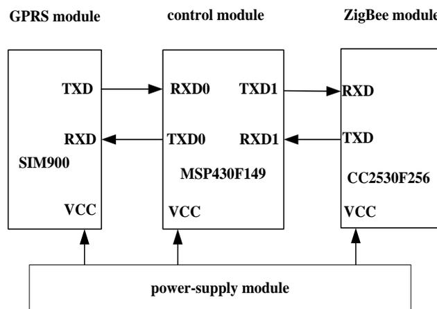
**Figure 2. Gateway Node Hardware Interface Circuit**
