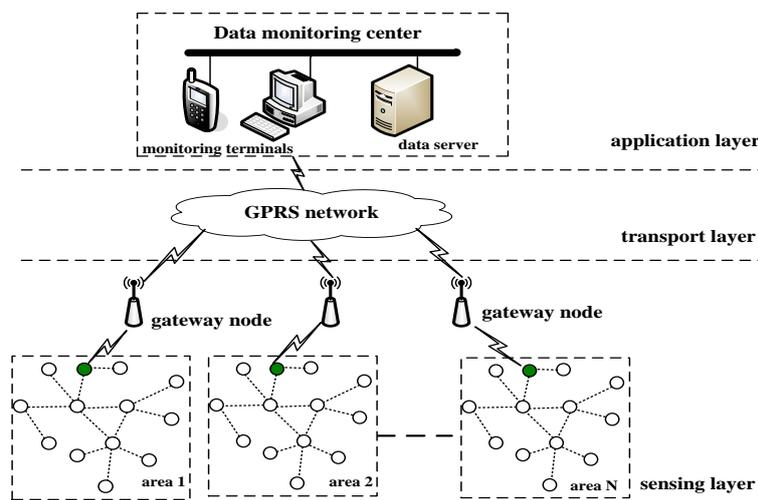
Figure 1. The Structure of System
