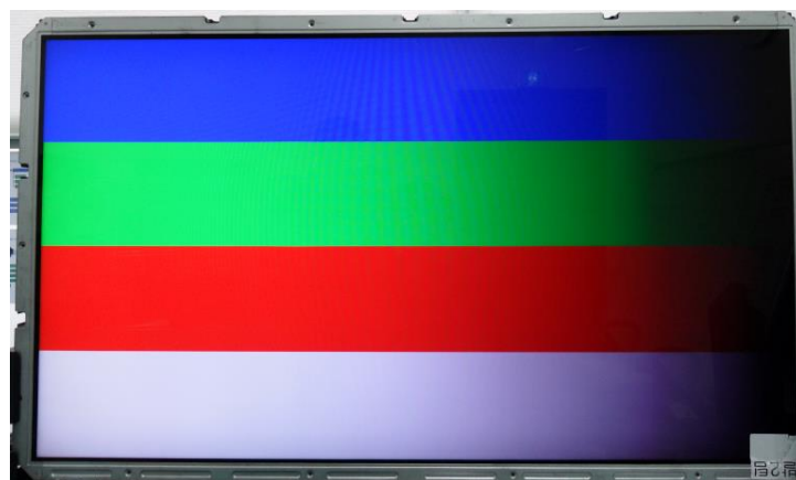
Figure 7. Photograph of an LCD TV Module with an LED Backlight Unit Operated By the Prototype Converter
