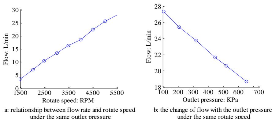
**Figure 4. The Relationship between the Flow with the Outlet Pressure And Speed**
