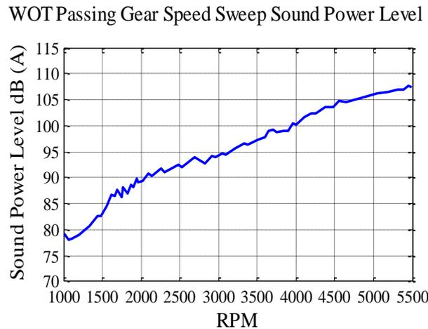
**Figure 2. The Noise Increased With the Speed Rise**
