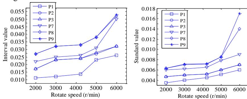
**Figure 5. Pump Intake Section, Outlet Section Monitoring Point Range Values at Each Speed**
