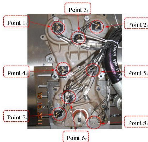
**Figure 1. Sensor and Testing Point Layout Diagram of Sample**
