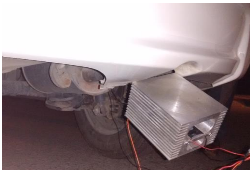
Figure 11. The ATEG Structure Attached to the Exhaust Pipe
