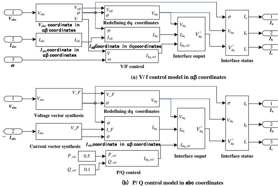
Figure 5. Integrated Simulation Model
