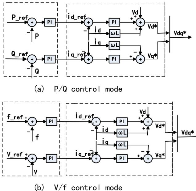
Figure 4. Control Mode of Microgrid
