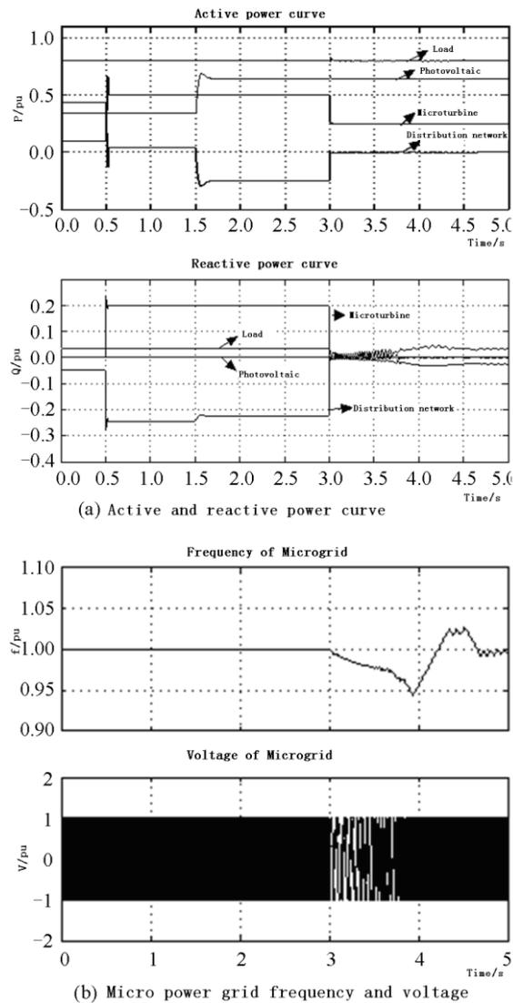
Figure 7. Simulation of the Discrete Mode
