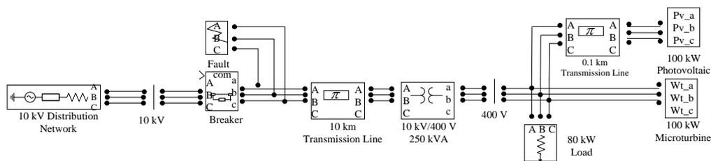
Figure 6. Microgrid Simulation System Diagram
