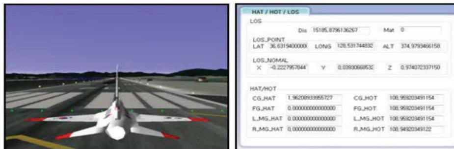
Figure 9. Identifying HOT, HAT, and LOS, Left : Aircraft Position, Right : Measured Values
