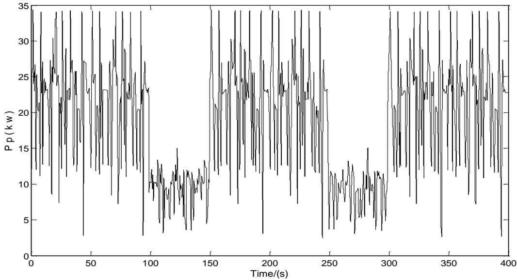
**Figure 5. Hydraulic Pump Output Power Curve**
