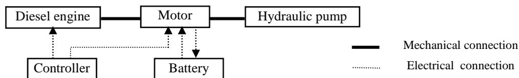
Figure 1. Parallel Hybrid Power System Structure
