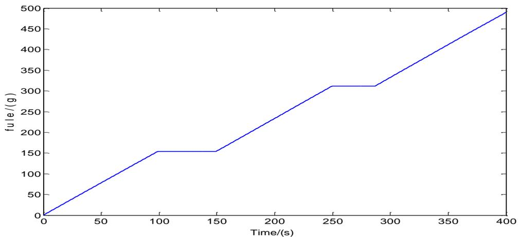
**Figure 10. Diesel Engine Fuel Consumption Curve**
