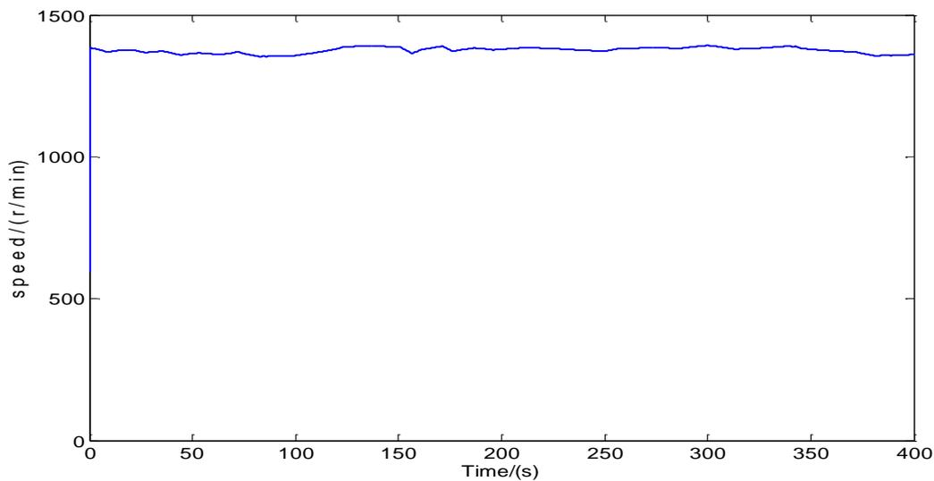
**Figure 9. Diesel Engine Shaft Rotate Speed Curve**
