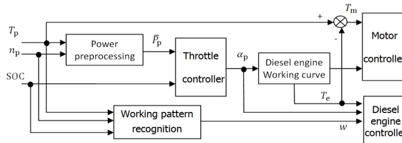
**Figure 2. Hybrid Power System Controller Structure**
