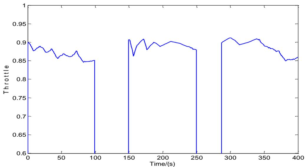
**Figure 8. Diesel Engine Throttle Opening Curve**
