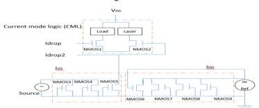
Figure 5. Laser Driver Circuit using Current Mode Logic
