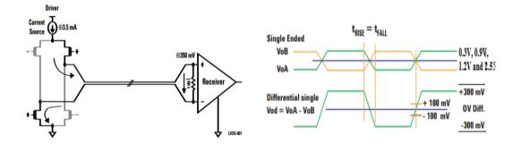
Figure 1. Diagram of LVDS Driver and Receiver Connected via Differential Impedance Media [7] Figure 2. The Lowered Voltage Swing Maintains High Speed and Consume Less Power [8]
