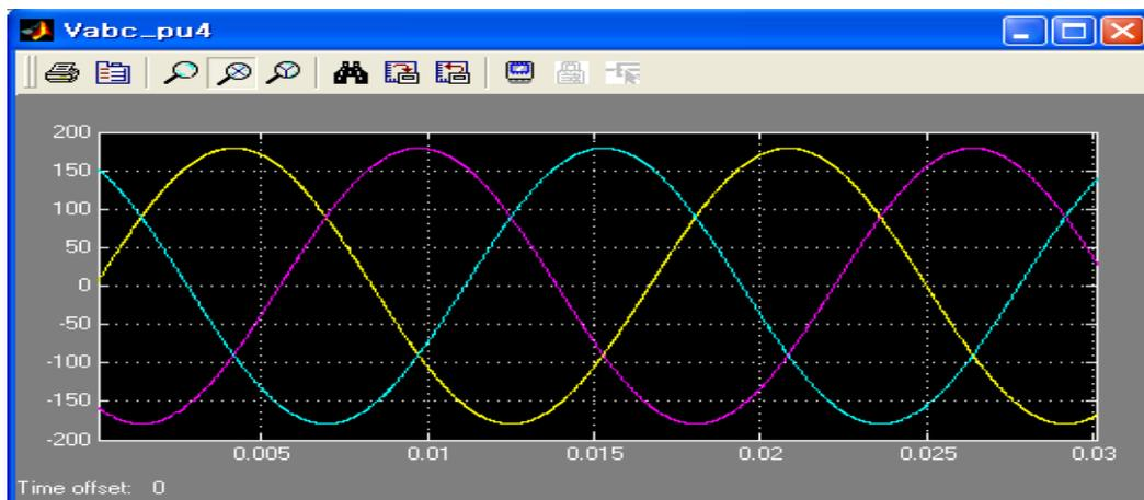
**Figure 11. The Secondary-Side Low Voltage Waveform at P4 of the Other Transformer Cross One Transformer for Carrier Signal of 290 kHz and 300 mA**
