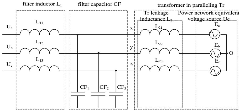
**Figure 2. Line-Side LCL Filter**
