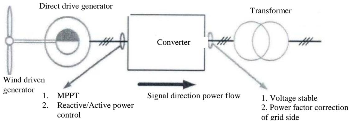
Figure 1. Structure of Wind Power System
