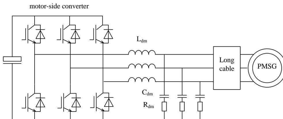
**Figure 5. A Du/Dt Filter Circuit of Generator-Side**
