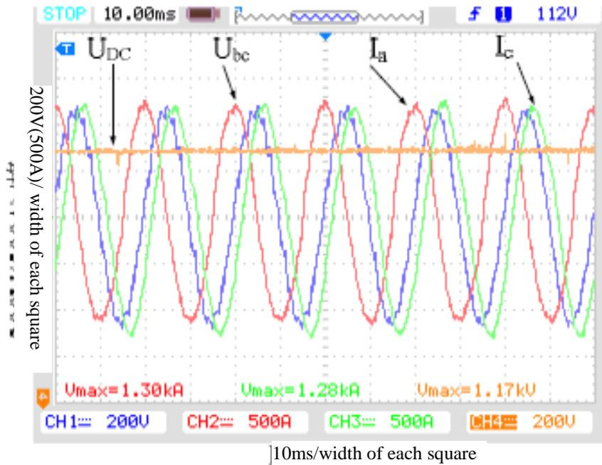
Figure 9. Waveform of the Line-Side When 1MW
