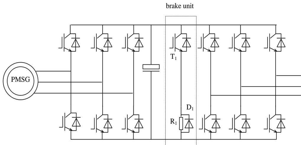
Figure 6. Brake Unit Structure
