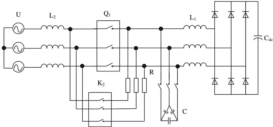
**Figure 7. Circuit of the Pre-Charge**
