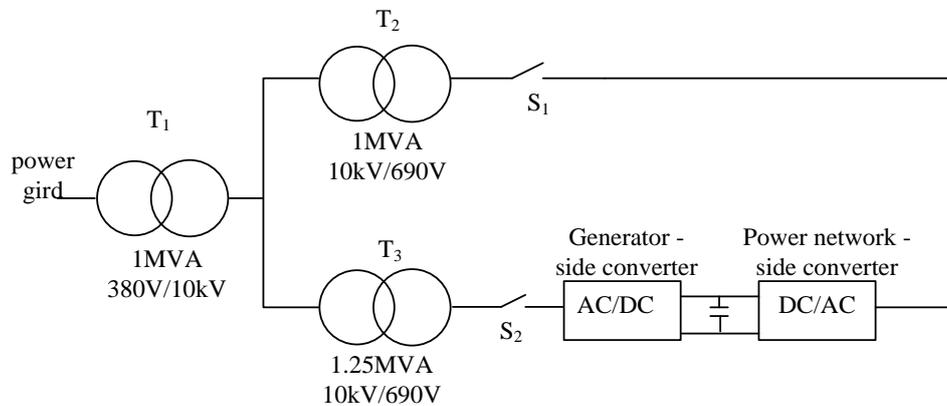
**Figure 8. Topology of Experimental Platform**
