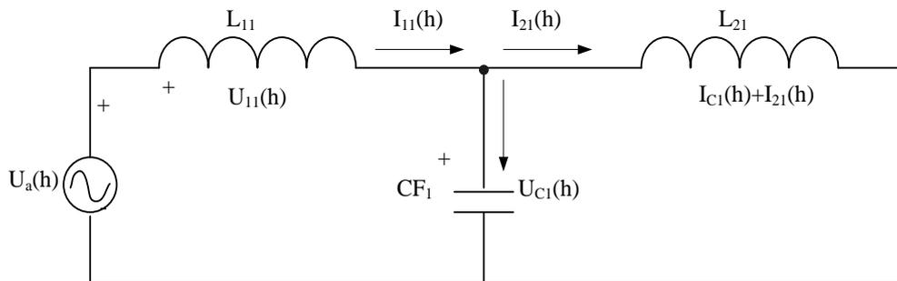
**Figure 3. Line-Side LCL Filter for One Phase**
