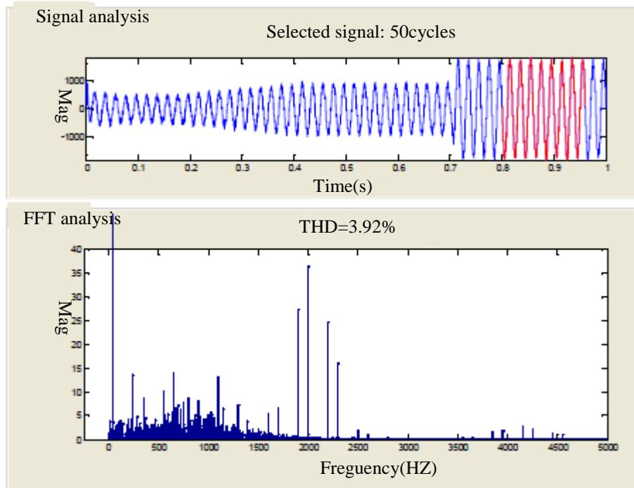
Figure 4. Current FFT Analysis of Line-Side
