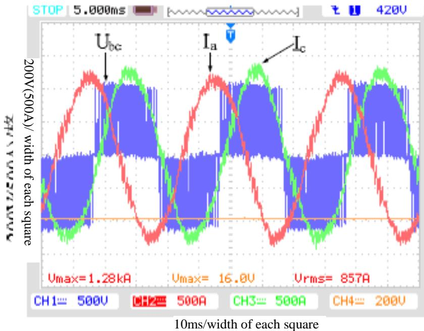
Figure 10. Waveform of Generator-Side Converter When 1MW
