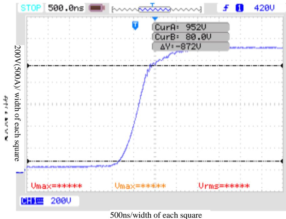
**Figure 11. Waveform of the Generator-Side Converter Line Voltage**
