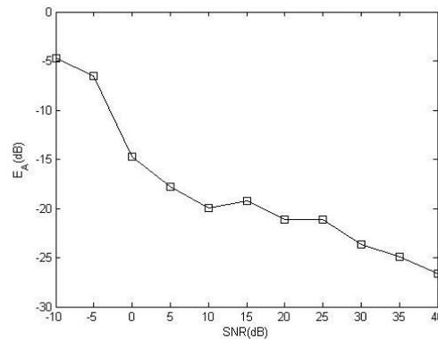
**Figure 2. The Matrix Estimation Error under Different SNR**
