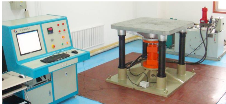
Figure 10. FCL Compression Testing Machine and Testing System
