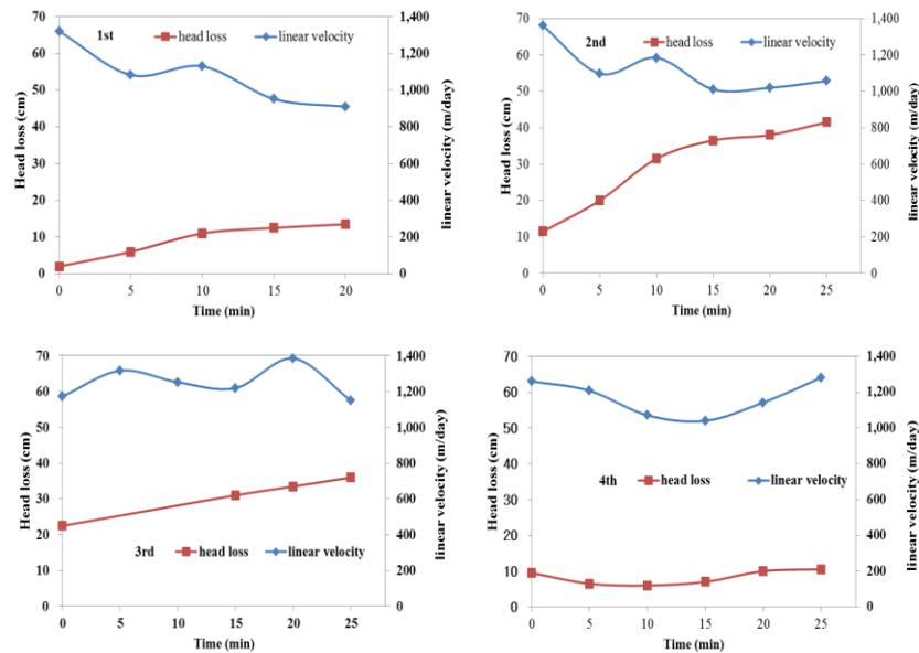
**Figure 6. Changes in the Head Loss and Filtering Linear Velocity by Short-Term Rainfall Event**
