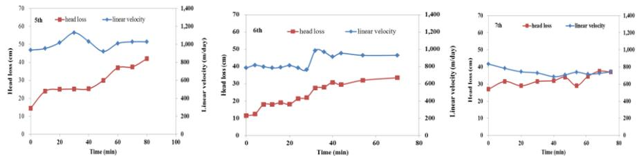
**Figure 8. Changes in the Head Loss and Filtering Linear Velocity by Long-Term Rainfall Event**
