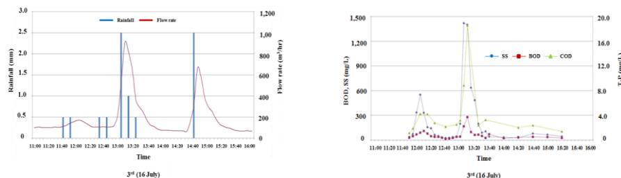
**Figure 5. Changes in the Flow Rate and Water Quality during Rainfall**
