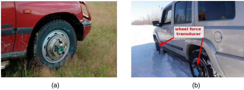
Figure 2. (A) Application of a Rotating Wheel Dynamometer (B) Application of Wheel Force Transducer
