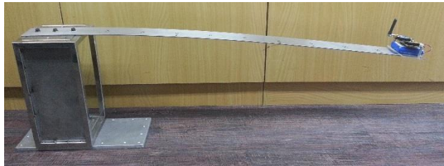
Figure 7. A Wireless Accelerometer on a Cantilever Beam
