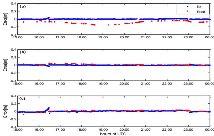
**Figure 11. Position Errors of Satellite Selection Method Based on SNR Fluctuation. (A) E Direction. (B) N Direction. (C) U Direction**
