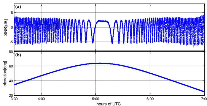
**Figure 4. (A) Fluctuation of GPS SNR Measurements Resulting from Multipath, (B) Corresponding Satellite Elevation Angles**
