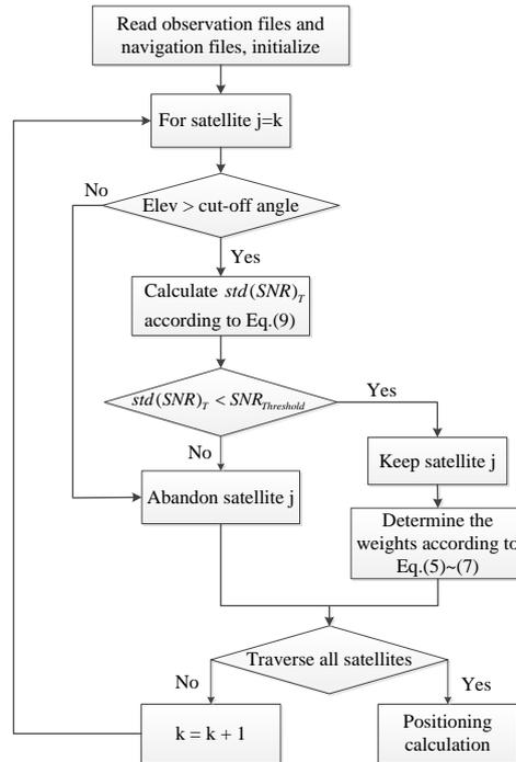
**Figure 9. Flow Chart of Satellite Selection Method Based on SNR Fluctuation**
