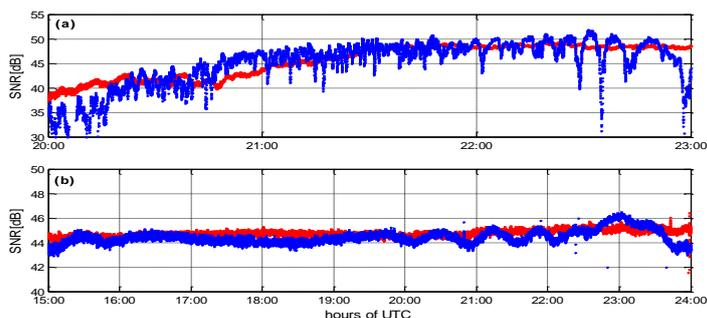
**Figure 7. Test Results of Real Observation Environment.(A) SNR of GPS Satellite, PRN3. (B) SNR of BDS Satellite, PRN3.**
