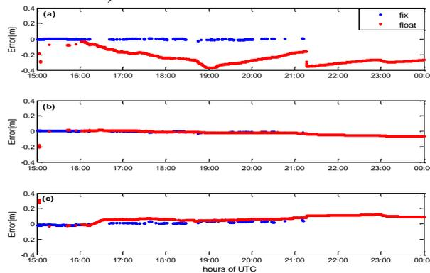
**Figure 10. Position Errors of Conventional Satellite Selection Method. (A) E Direction. (B) N Direction. (C) U Direction**
