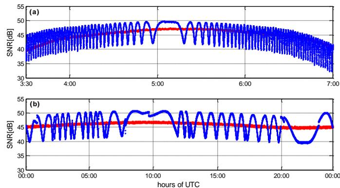
**Figure 3. Test Results of Simulator. (A) SNR of GPS Satellite (MEO), (B) SNR of BDS Satellite (GEO)**
