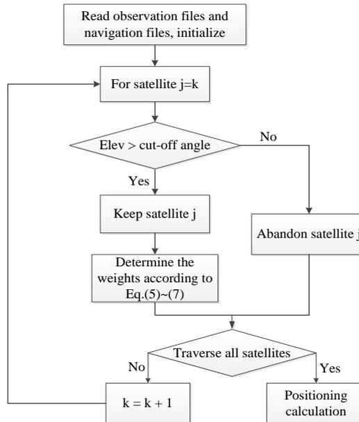
**Figure 8. Flow Chart of the Conventional Satellite Selection Method**
