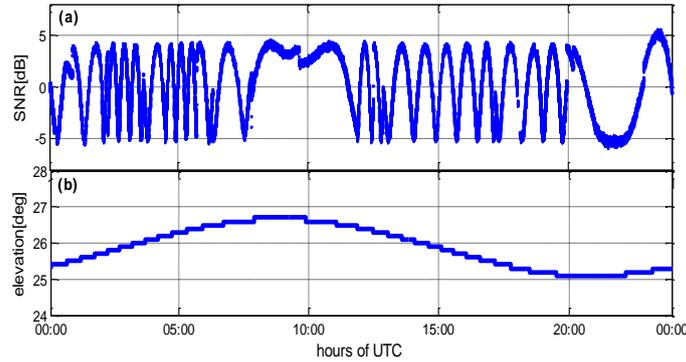
**Figure 5. (A) Fluctuation of BDS SNR Measurements Resulting From Multipath, (B) Corresponding Satellite Elevation Angles**
