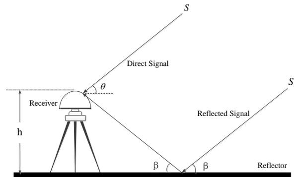
**Figure 1. Schematic Diagram of Multipath Phenomenon**
