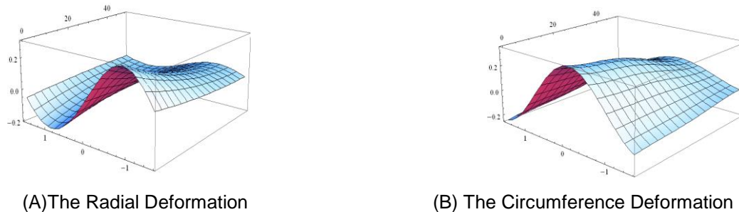
Figure 10. Displacement of the Axis When the Temperature is 40 Centigrade under the Working Condition
