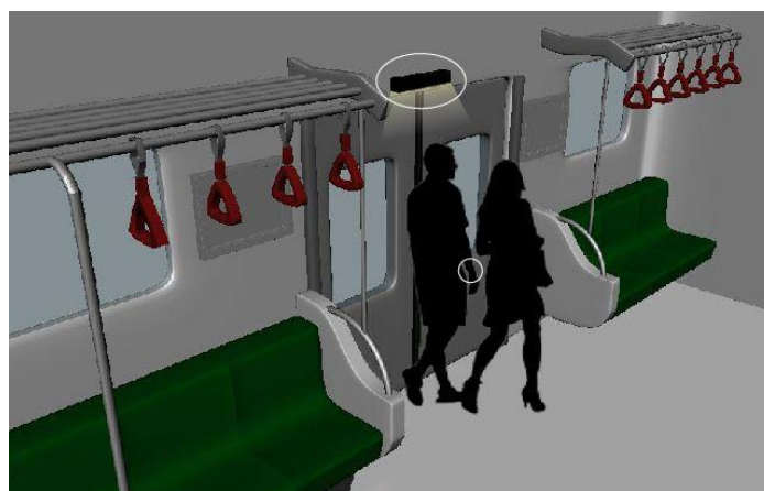
Figure 5. RFID/NFC Sensor Installed at the Entrance to a Car Sensing a Smart Phone or Smart Watch Including an RFID/NFC Tag Carried by a Passenger
