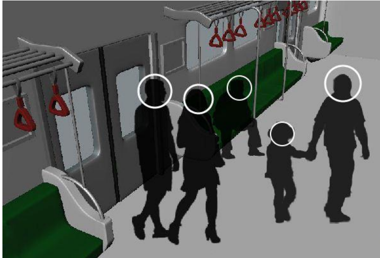
Figure 4. Recognition of the Heads of the Passengers using Head Colors
