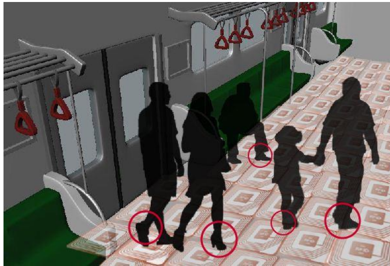
Figure 6. RFID/NFC Sensors Installed on the Floor of the Car Sensing Smart Shoes or Antenna Bands Including RFID/NFC Tags Worn by the Passengers
