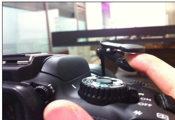
Figure 7. The Capturing Part of the Heart-Rate Pulse Printer Using Finger-Tipped Pulse Sensor
