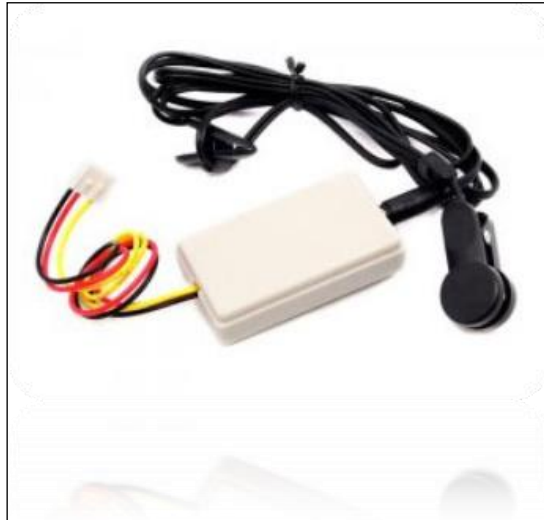
Figure 6. Ear/Finger-Clip Heart-Rate Sensor
