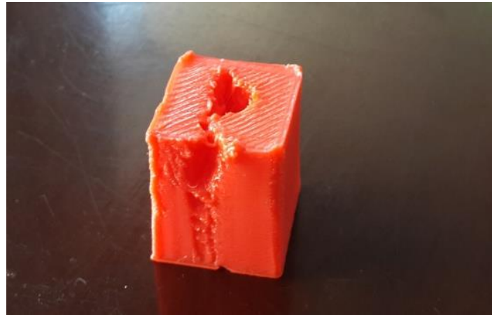
Figure 6. A Test Sample Which Heating Temperature Is 215 °C, the Throat Diameter is \Phi 18mm and the Thickness is 0.3 Mm in Natural Convection Coefficient of 180 W/(M 2 ·°C)
