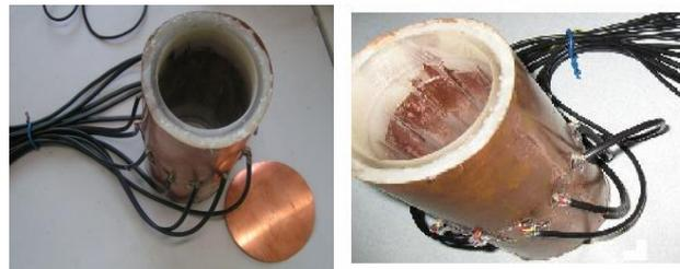
**Figure 4. Structure of Capacitance Sensor**
