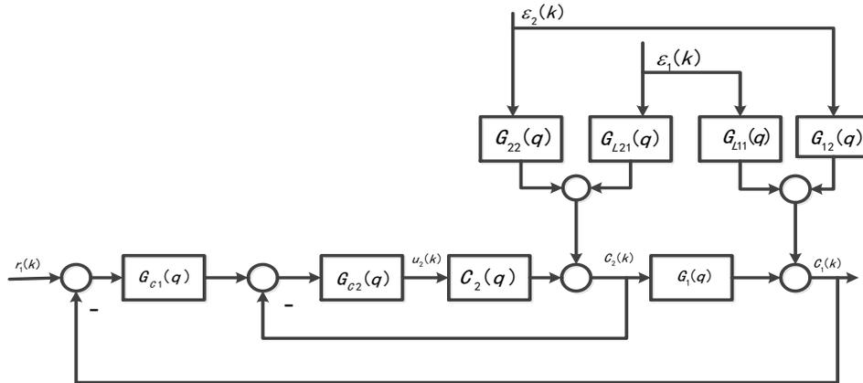
Figure 4. Cascade Control System Block Diagram
