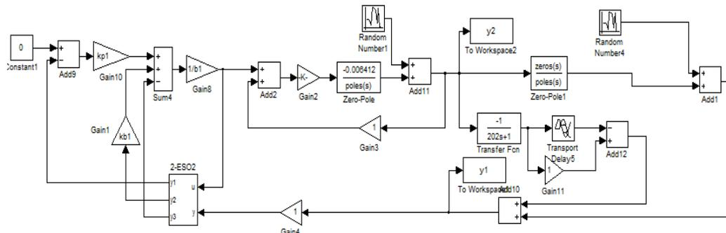
**Figure 5. 37% Load Under Smith ADRC - Proportional Cascade Control System**
