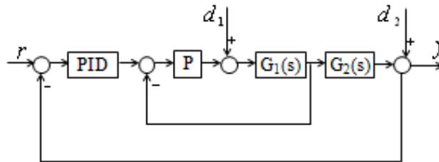
Figure 1. Cascade Control System Diagram
