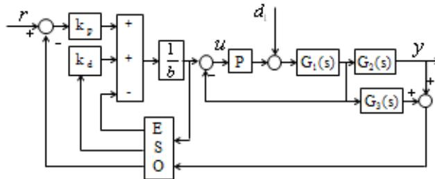
**Figure 3. Smith ADRC Cascade System Block Diagram**
