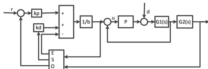
Figure 2. ADRC Cascade System Block Diagram
