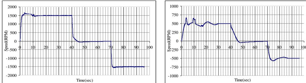
(a) Setpoint changed from 0 rpm to 1500rpm, from 1500rpm to 0rpm, and from 0rpm to -1500rpm
