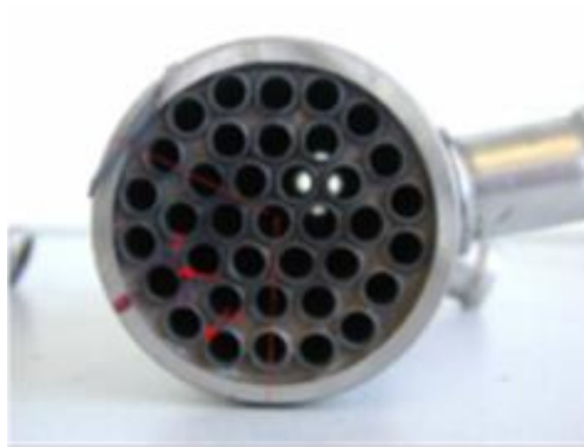
Photo 2. Crack Locations on Header
