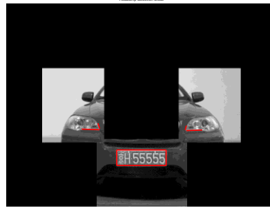
Figure 6. The Front License Plate Location and Headlight Feature Points of the Model Car
