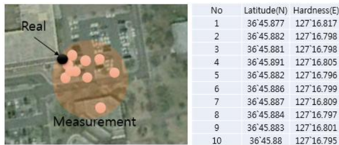
Figure 1. GPS distance errors in a NLOS environment
