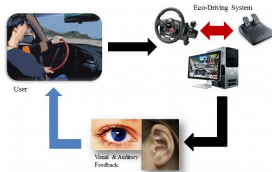
Figure 1. Overview of the proposed virtual eco-driving training simulator
