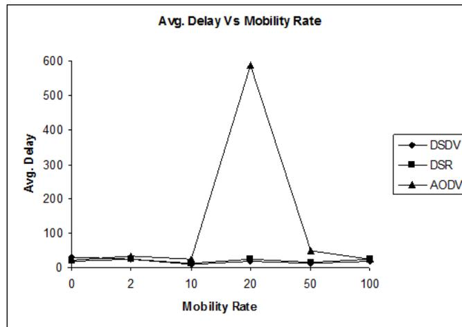
**Figure 11. The average delay versus the mobility rate for 10 active sources, area 700 x 700**
