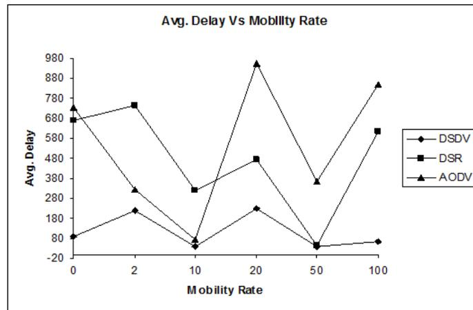
Figure 13. The average delay versus the mobility rate for 30 active sources, area 700 x 700
