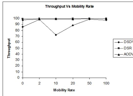
**Figure 2. The throughput versus the mobility rate for 10 active sources and area 500 x 500**
