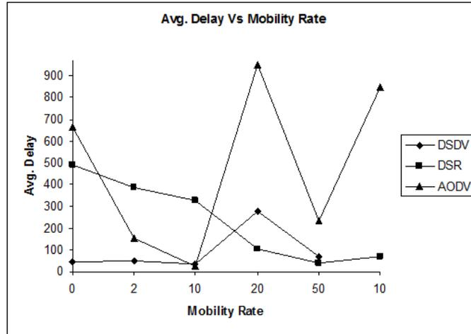
Figure 12. The average delay versus the mobility rate for 20 active sources, area 700 x 700
