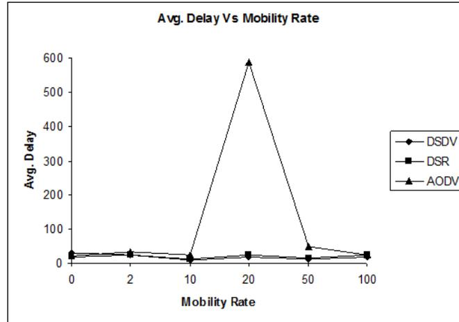
**Figure 10. The average delay versus the mobility rate for 30 active sources, area 500 x 500**
