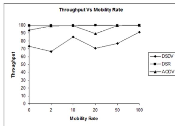
Figure 5. The throughput versus the mobility rate for 10 active sources and area 700 x 700
