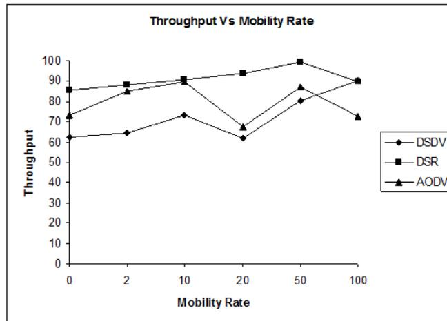
**Figure 7. The throughput versus the mobility rate for 30 active sources and area 700 x 700**
