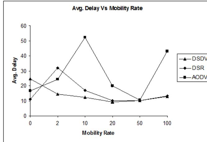
**Figure 8. The average delay versus the mobility rate for 10 active sources and area 500 x 500**
