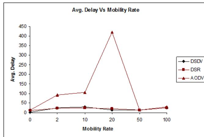
**Figure 9. The average delay versus the mobility rate for 20 active sources and area 500 x 500**
