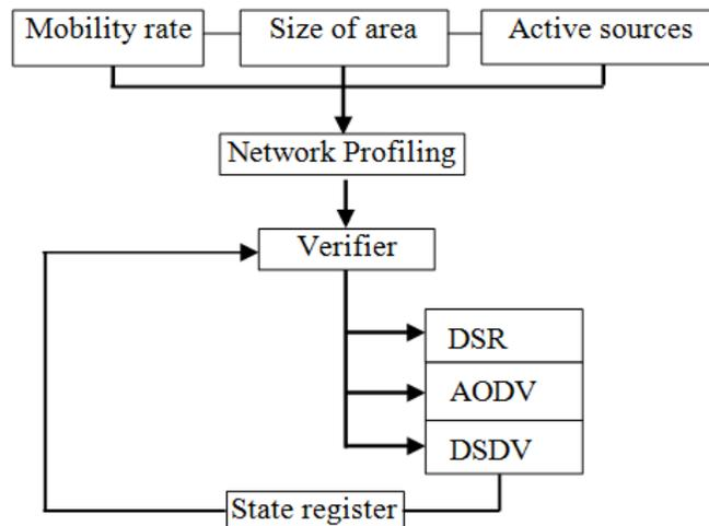
**Figure 1. Proposed architecture with three routing protocols: DSR (Dynamic Source Routing), AODV (Ad Hoc on Demand Distance Vector Routing and DSDV (Destination Sequenced Distance Vector).**
