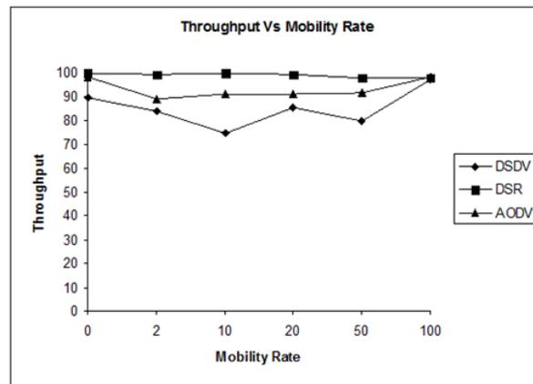
Figure 4. The throughput versus the mobility rate for 30 active sources and area 500 x 500
