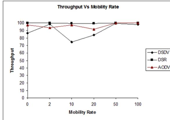
Figure 3. The throughput versus the mobility rate for 20 active sources and area 500 x 500
