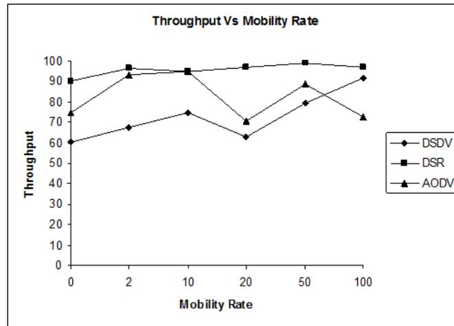
**Figure 6. The throughput versus the mobility rate for 20 active sources and area 700 x 700**
