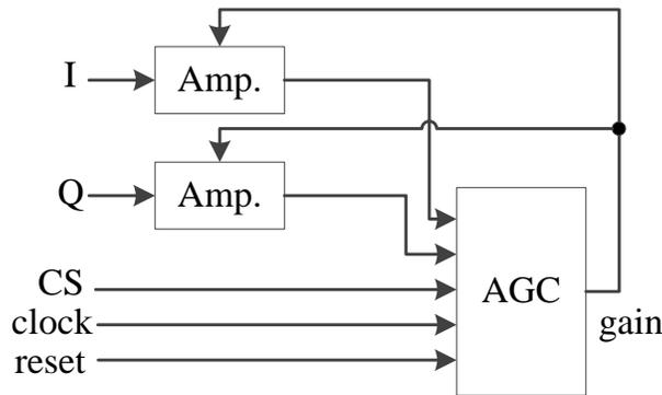
**Figure 1. Block diagram of digital equivalent system for gain control**
