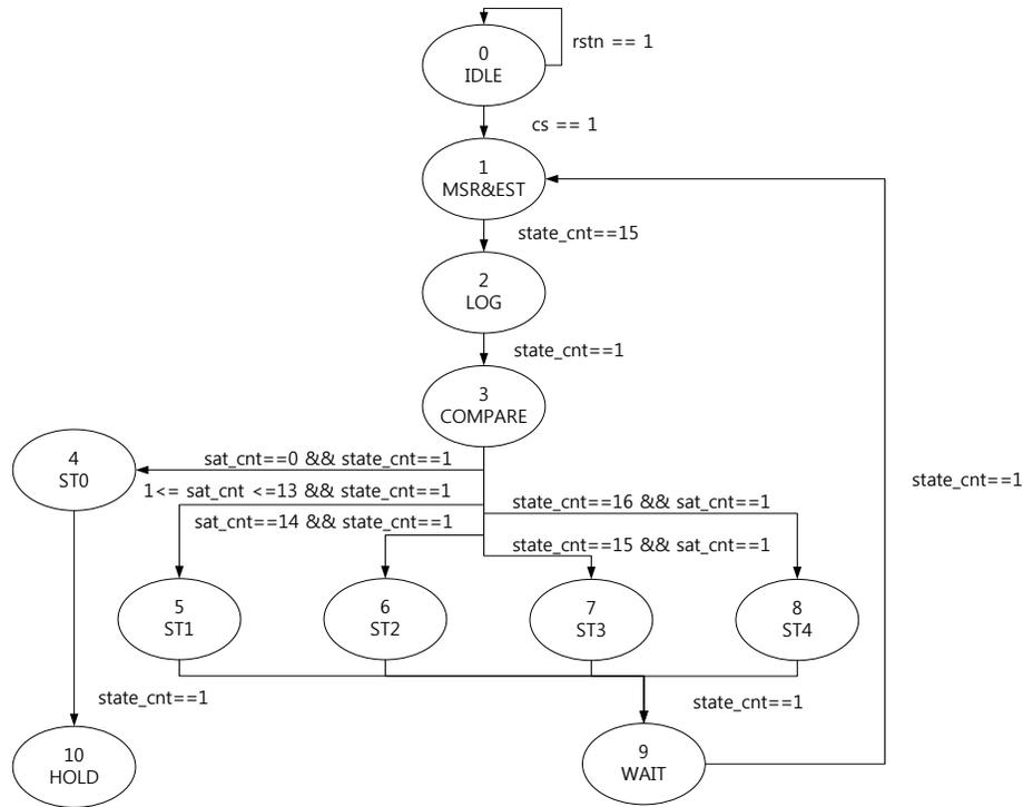
**Figure 2. State diagram for the AGC with multiple gain loops**
