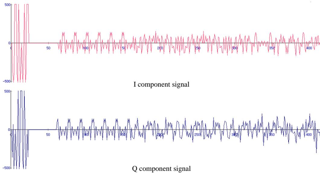
**Figure 4. Controlled waveforms obtained with FPGA level experiment (70dB input)**
