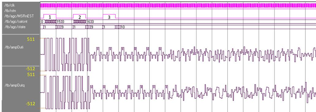
**Figure 5. Controlled waveforms obtained with RTL simulation (140dB input signal)**
