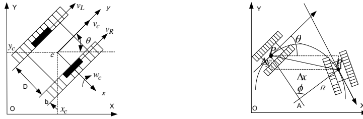
(a) The position and attitude of the robot (b) The sketch map of the robot move round
