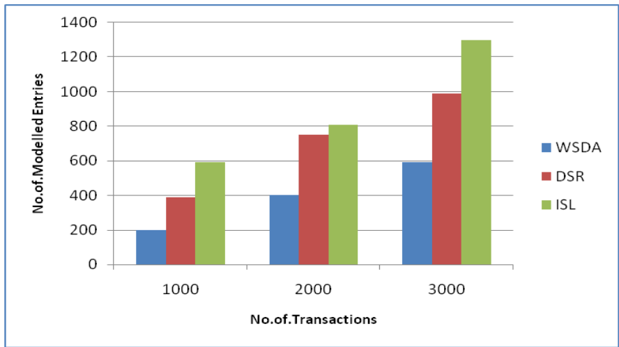
Figure 4.2 Performance Comparison of WSDA with DSR and ISL for Modified Entries with Number of Transactions
