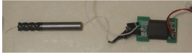
Figure 5. The Photo of Thermocouple Connect to Guest Through one Tool Coolant Hole
