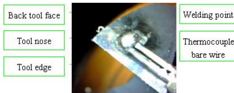
Figure 2. Welding Photograph of Thermocouple and Tool Flank
