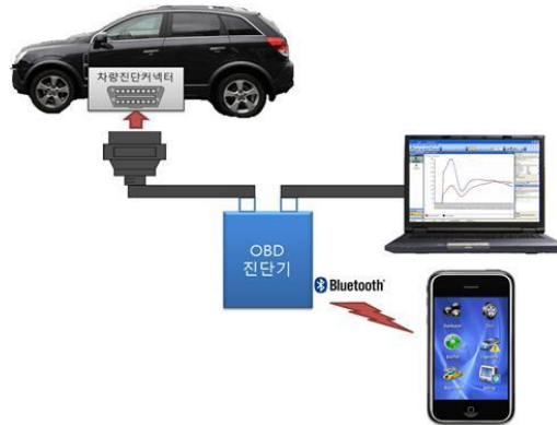
Figure 3. Diagnosis schematic diagram using the Bluetooth network
