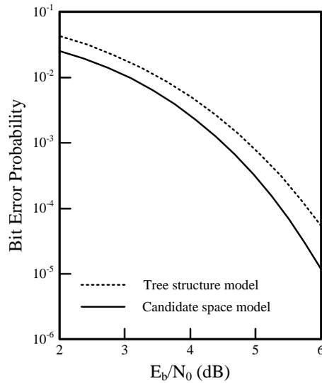
Figure 1. Bit error probability of (63,30) BCH code
