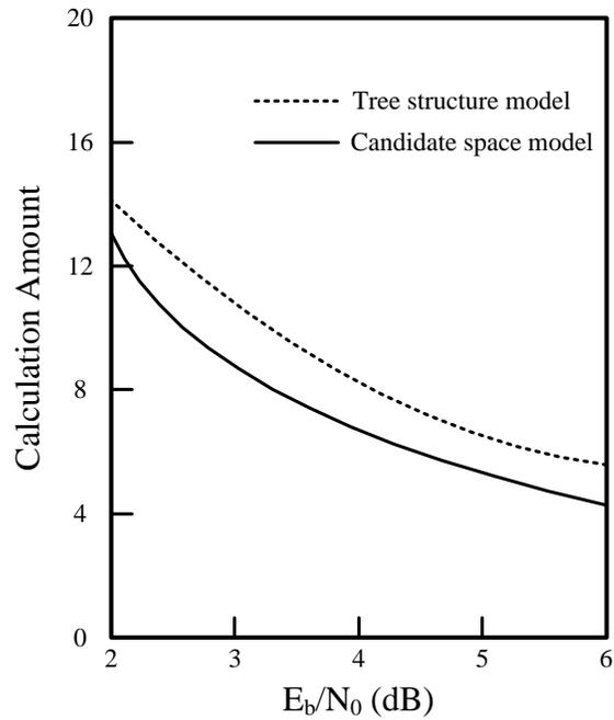
Figure 6. The calculation amount of (63,30) BCH code
