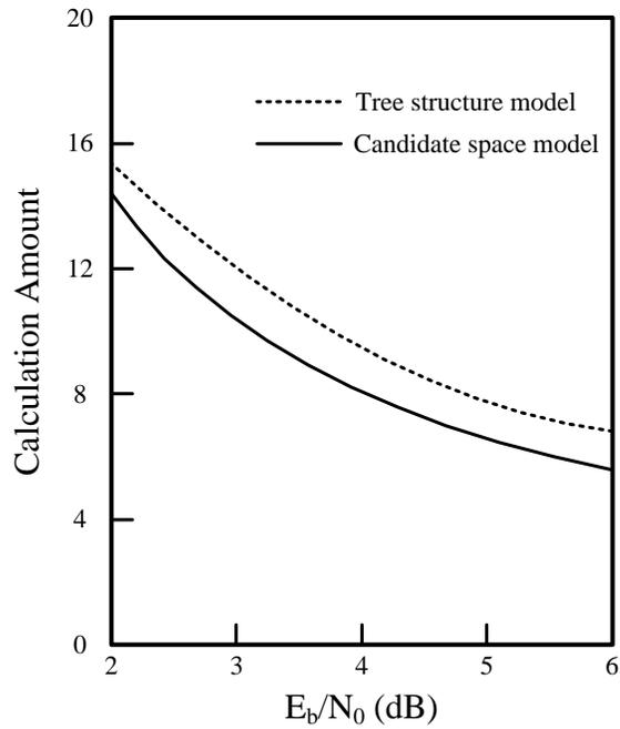
**Figure 8. The calculation amount of (64,42) RM code**
