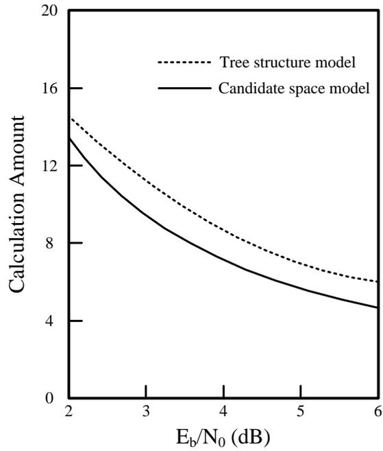
**Figure 7. The calculation amount of (24,12,8) extended Golay code**
