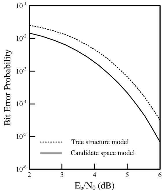
**Figure 4. Bit error probability of (128,99) extended BCH code**
