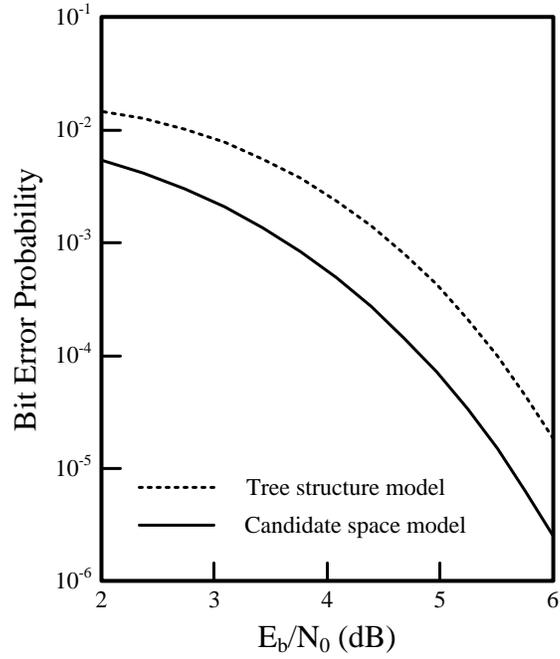
Figure 5. Bit error probability rate of (128,64) extended BCH code
