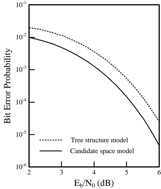
**Figure 3. Bit error probability of (64,42) RM code**
