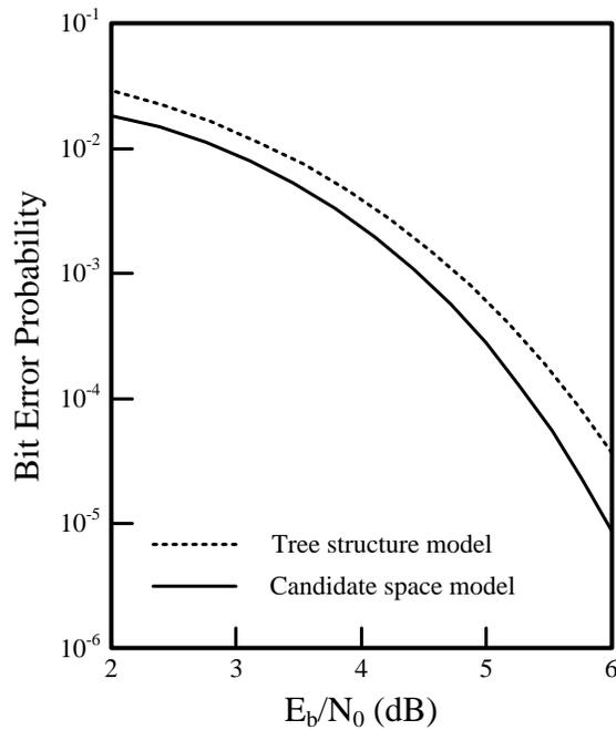
Figure 2. Bit error probability of (24,12,8) extended Golay code
