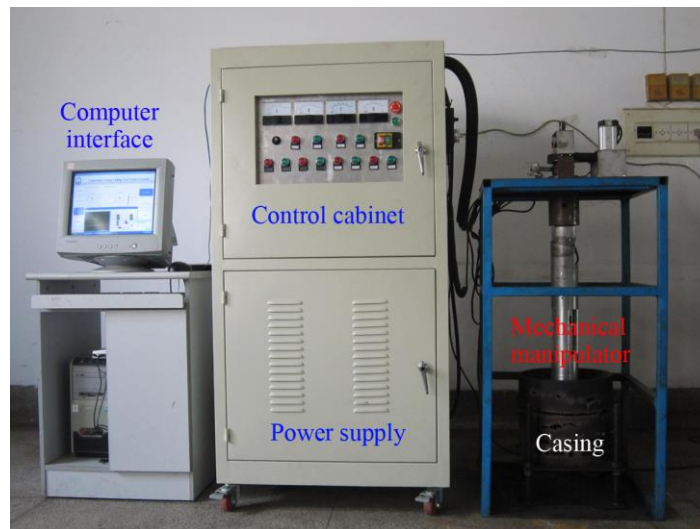
Figure 6. Prototype of the cutting robot in laboratory
