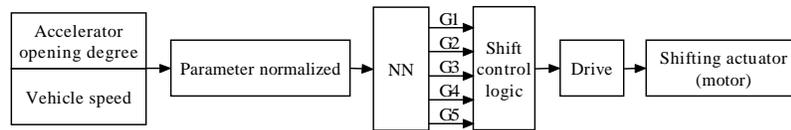
**Fig. 6. The best stalls do and shift control logic diagram**
