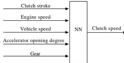
**Fig. 7. Clutch neural network input and output**
