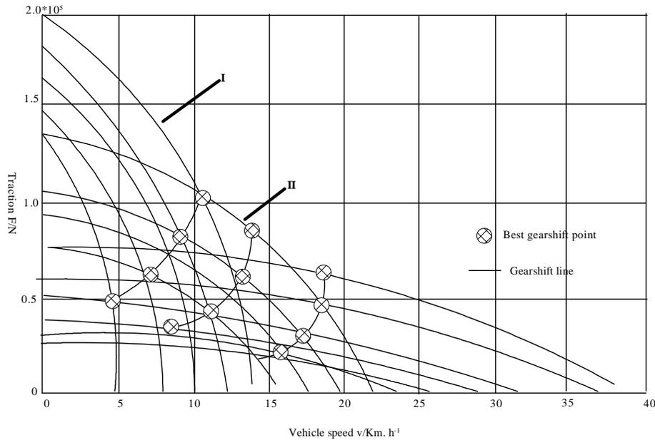
**Fig. 1. Advance-speed traction characteristics**
