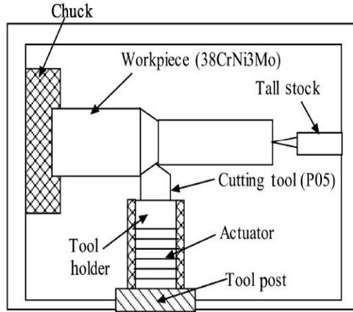
Figure 1. Metal cutting machine [5].
