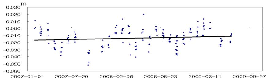
**Figure 5. Movement of Barton Peninsula - Ellipsoidal height**
