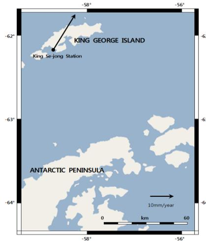
**Figure 6. Movement Direction and Velocity of Barton Peninsula**
