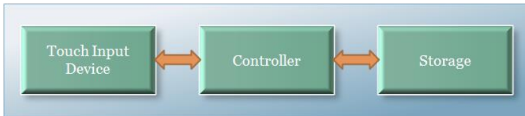
Figure 6. An example of a block diagram of a mobile device in which a method of recognizing a pointer control command based on finger motion is implemented
