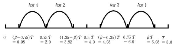
**Figure 4. Gait diagram with  $\beta = 0.76$  and  $T = 8$  sec.**
